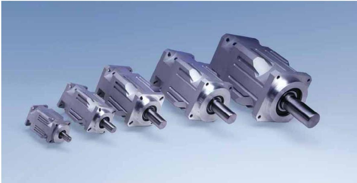
Servo gears of the AP and HP series: one-stage and two-stage planetary gears with low torsional backlash and high torsional rigidity, or hybrid gears, comprising a precision planetary gear and a preceding spur gear.
